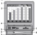
**1. Power indicator**Red LED turns ON when the power is supplied.
