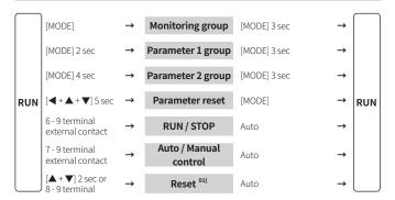
01) In the event of system anomalies and alarms, RESET input restarts the power controller. (parameters are not reset.)
