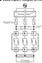
01) When connecting noise filter and capacitor, it is appropriate for EMC.
